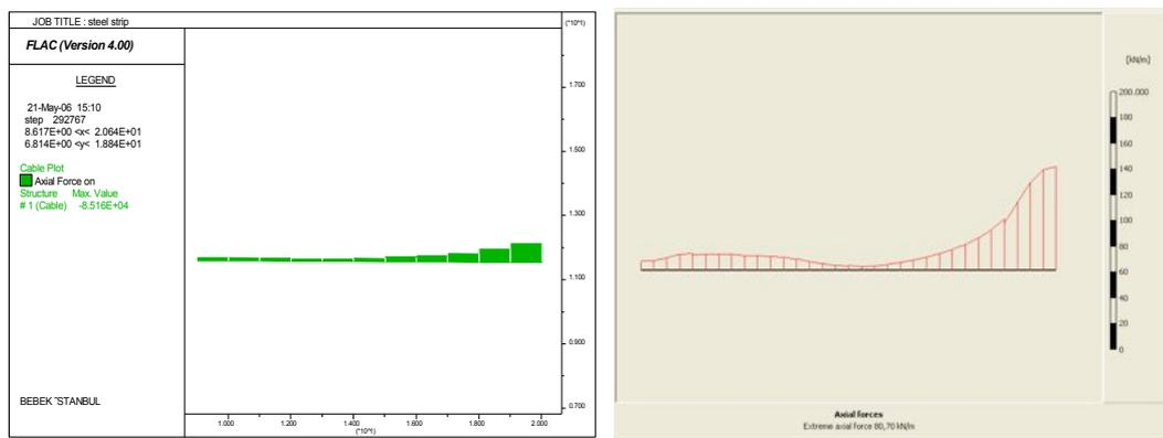
**Figure 6.** (FLAC and PLAXIS Stresses at the Lowermost Strips, Seismic Condition).
