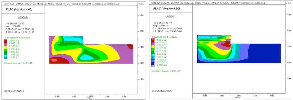
Figure 2. (FLAC Analysis Results Static Condition).
