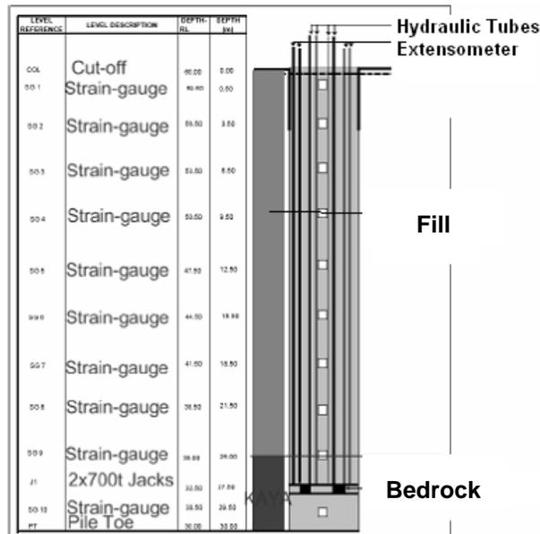
Figure 7. Configuration of Testing, ZETAS(2009).
