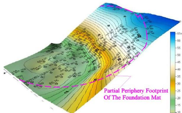
Figure 3. Bedrock Surface under the Foundation Mat
