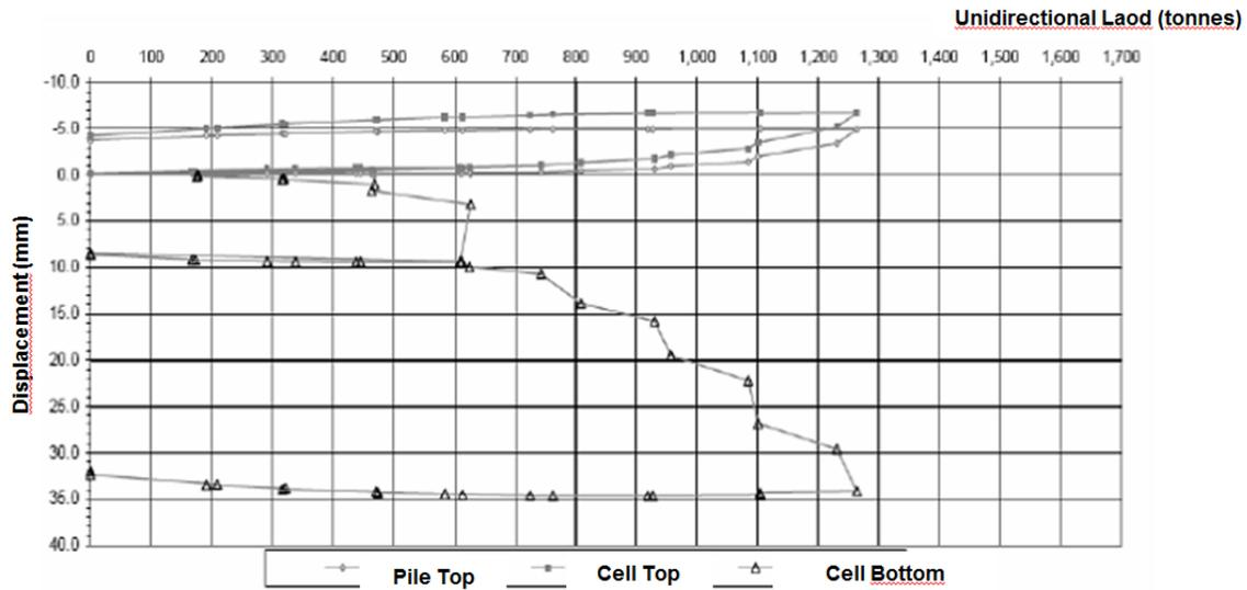
Figure 8. Load vs. Vertical Displacements, ZETAS(2009).
