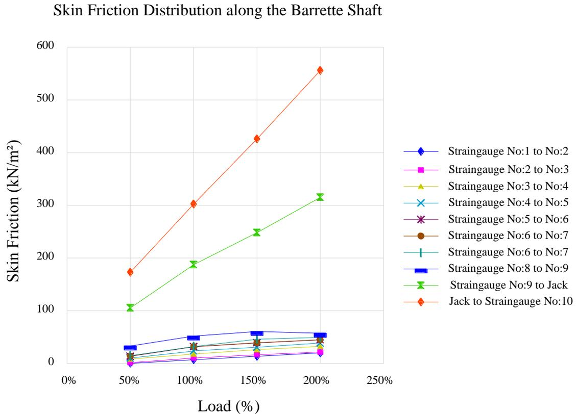
Figure 10. Unit skin friction vs. load (% of service load), ZETAS (2009).
