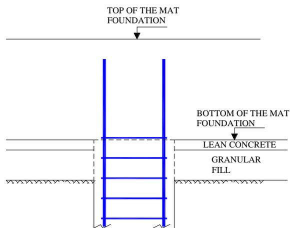
Figure 6. Typical Section for Barrette and Mat Foundation (ZETAS, 2009)
