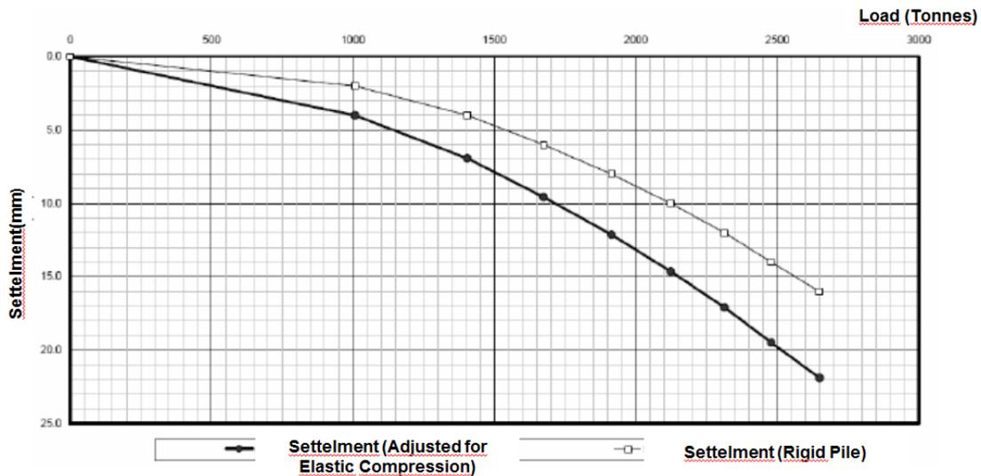
Figure 9. Load vs. Vertical Displacement, ZETAS(2009).
