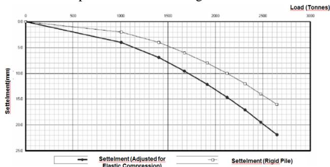
Figure 2. Load vs. Vertical Displacement, (Durgunoglu, 2013)
