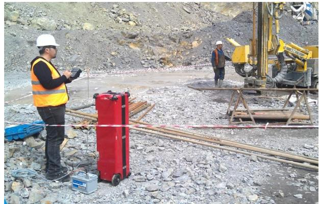
Figure 7 – Application of High Pressure Pressuremeter (HyperPAC) in Investigation Site.
