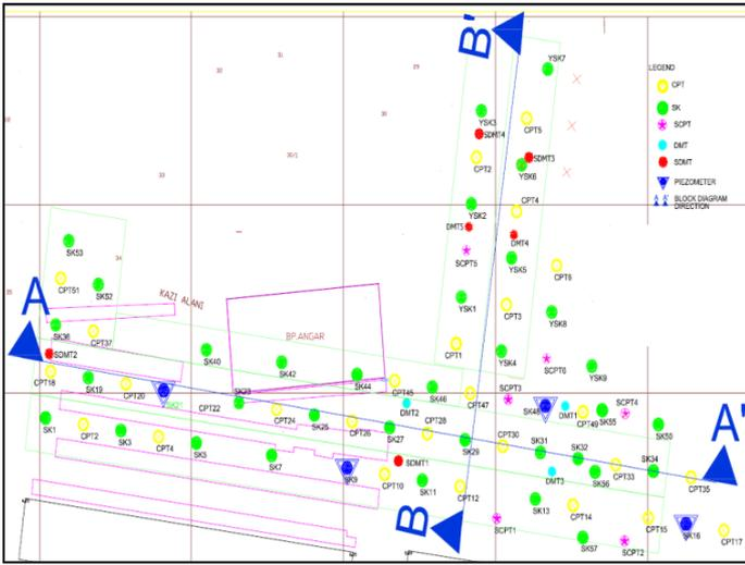
Figure 6 – Soil Investigations Layout Plan
