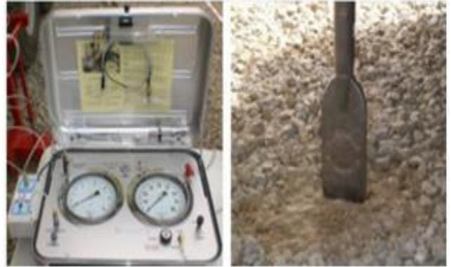
Figure – 5 Marchetti Dilatometer blade and control unit.
