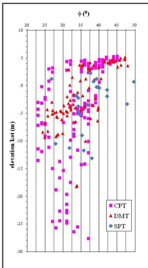
Figure 9 – Variation of internal friction angle with elevation
