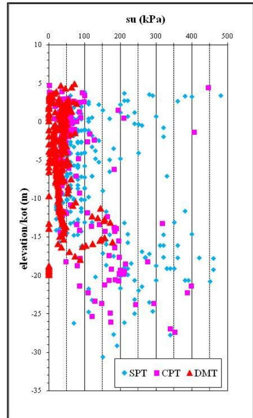
Figure 10 – Variation of undrained shear strength with elevation
