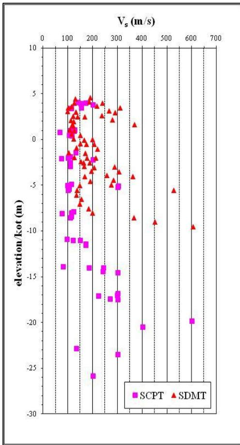
Figure 11 – Variation of shear wave velocities with elevation
