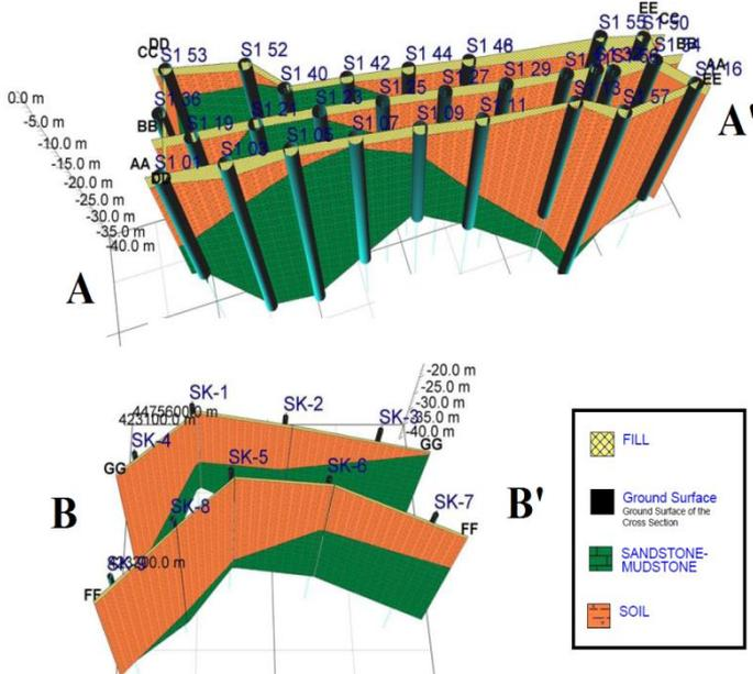
Figure 7 – A-A' and B-B' Block Diagram according to boreholes
