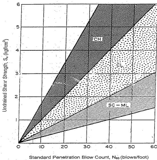
Figure – 1 Relationship between standard penetration blow count, N and undrained shear strength ( $s_u$ ), (after Sowers, 1979)
