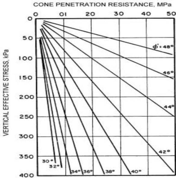
Figure – 4 Proposed correlation between cone bearing and peak friction angle (Robertson and Campanella, 1983)
