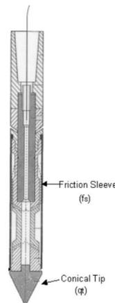
in load cells that record the end bearing stress ( $q_c$ ), and friction sleeve stress ( $f_s$ ). Readings are obtained at every 2.0cm depth. In seismic tests to measure shear wave velocities ( $v_s$ ) special seismic cones were employed, SCPT.
