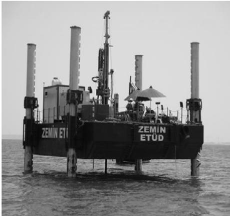
Figure 1. Zemin Etüd Jack-up Barge
