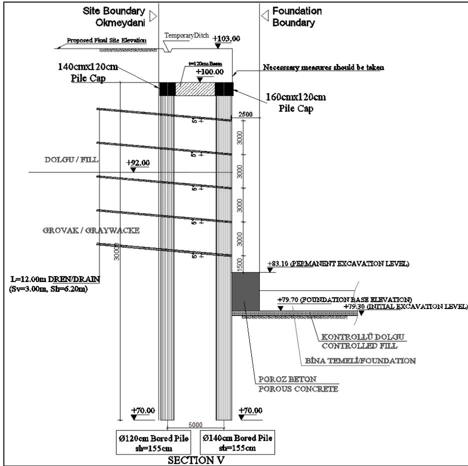
Figure 1 A Typical Section of the Preferred Retaining System Alternative
