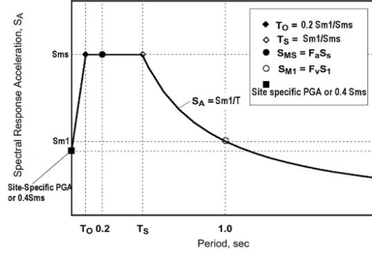
Figure 2. Standard Shape of the Response Spectrum (NEHRP, 2003)
